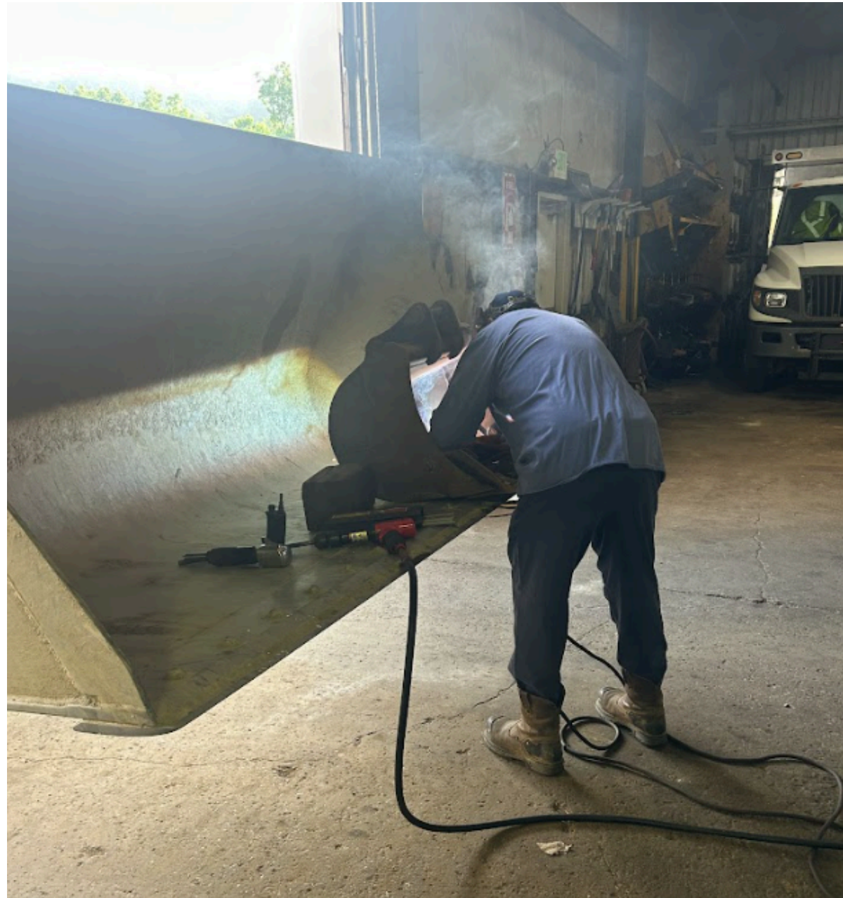
Repairing the bucket for the excavator
