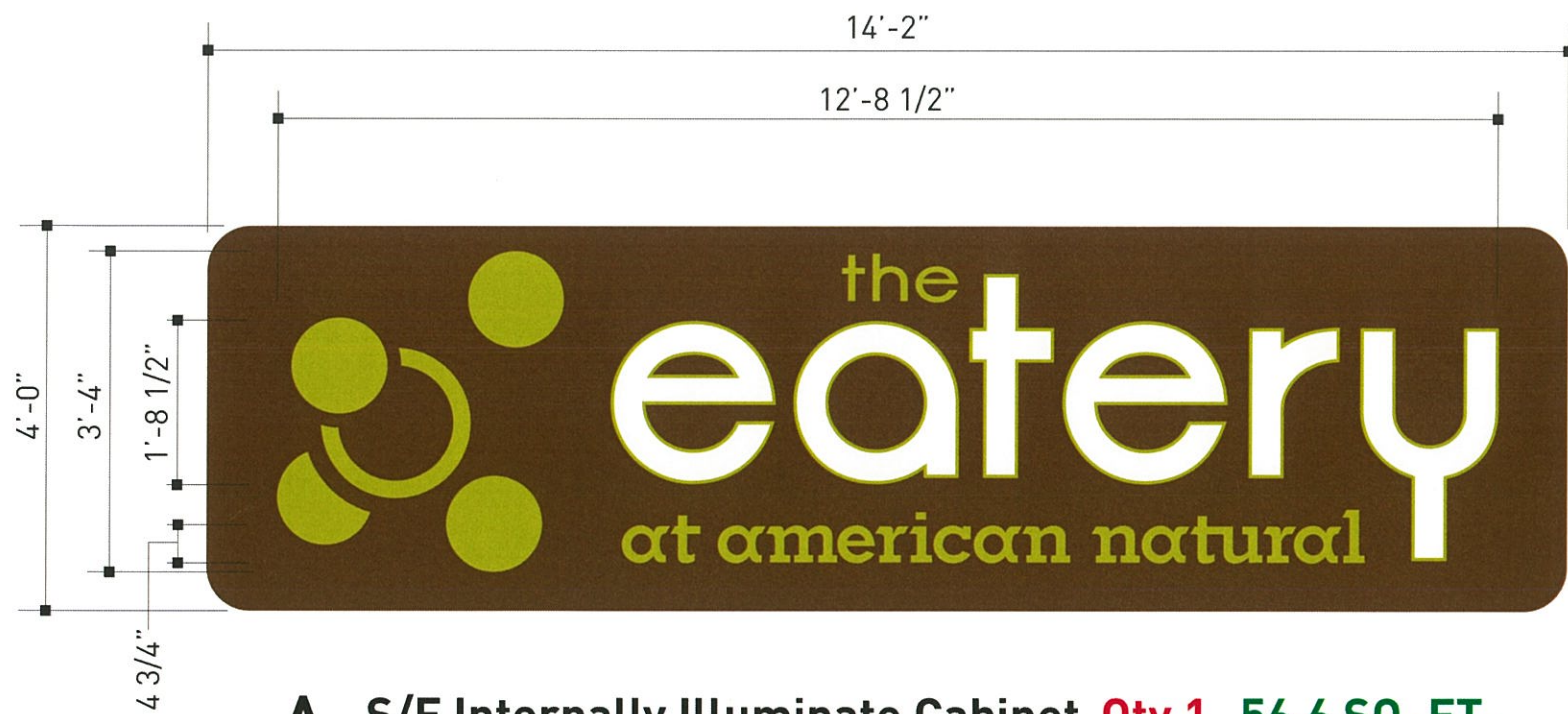
A S/F Internally Illuminate Cabinet Qty 1 56.6 SQ. FT. Scale: 1/2" = 1'-0"
